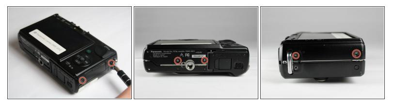
Using a Phillips #00 screwdriver, remove six 2.69mm, silver screws located on the two short sides of the camera and the bottom side.
