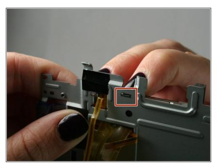
• Using your fingers, push down on the small, metal hooks that are a part of the metal cover and attach on top of the LCD screen.
