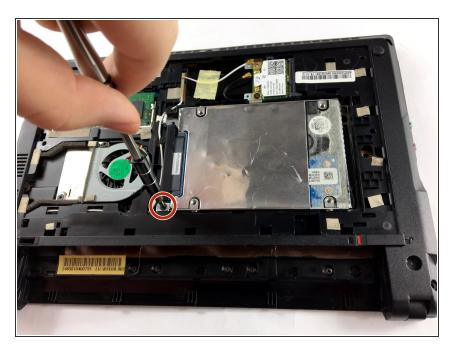
Using a Phillips #0 screwdriver, remove the indicated M2x2mm screw.
