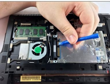
Use a plastic opening tool and slide the hard disk drive away from its port.
