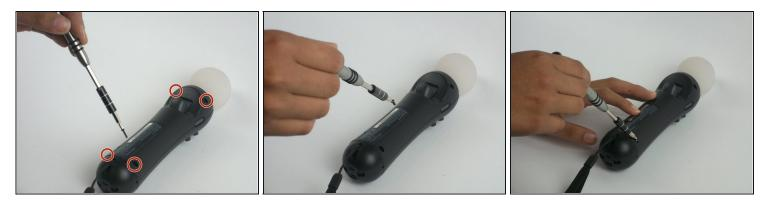
• Using a Phillips #0 screwdriver, remove the four 10mm screws located on the back of the device.
