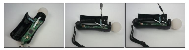
• Remove the five 1.2 mm screws from upper portion of the controller.
