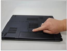
Slide the locking switch to the left to release the battery.
