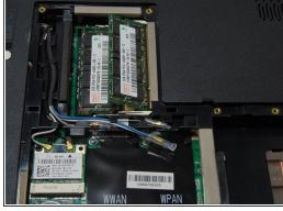
Press the tabs outwards to release the tabs. The memory stick is spring loaded and will be released at an angle.
