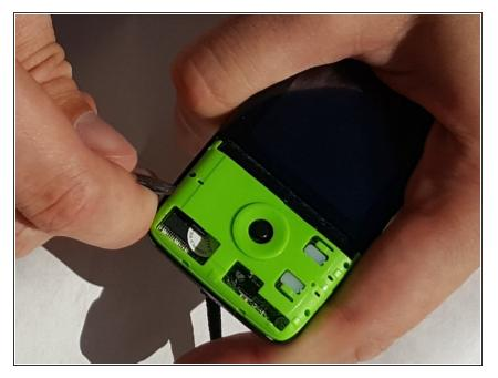
Find the groove around the outside of the green section. Use an ESD safe spudger to slowly lift the plastic panel up.
