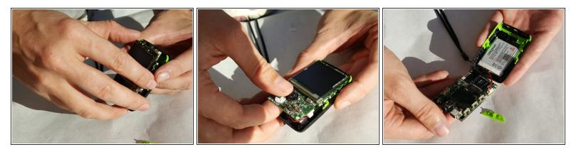
• Pull up on the motherboard and display. It is glued to the base so it will require a little force. Be careful though, as the board is fragile.
