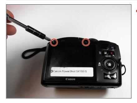
• Remove the two 2mm screws above the screen using the size J000 screwdriver.
