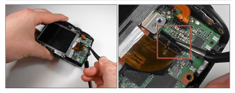
(i) There is a black flex ribbon lock that must be lifted and unlocked with your tweezers before this flex ribbon will detach.
