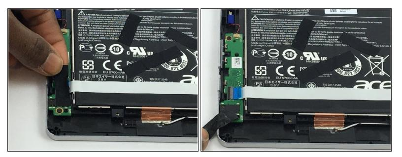
• Remove the tape to expose the left side of the ZIF connector.
