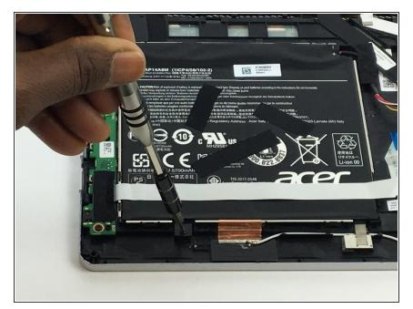
Use your screwdriver with the Phillips PH000 attachment to unscrew the single 4mm screw that holds the battery to the base plate.
