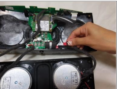
Remove the speaker wires from the motherboard by pinching the plastic tab at the end of the cable and pulling towards you.
