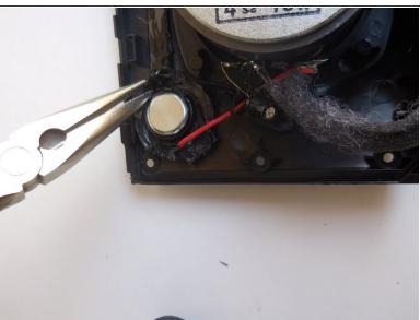
Remove both the black and red wires with pliers
