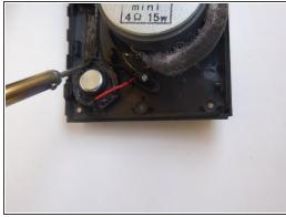
Solder the black plastic encasing the red and black wires.
