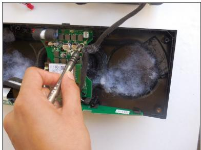
Unscrew 1.2 cm Torx security screw, holding the silver circle connector, to disconnect the wire from the speakerboard to the motherboard
