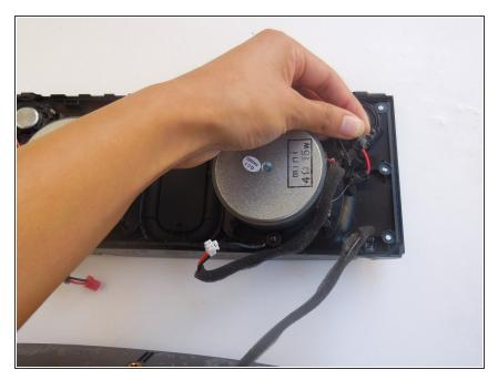
Remove the black putty from the speaker wires at both ends of the speaker board.
