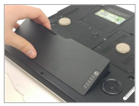
Remove the battery in to order avoid damaging internal components.
