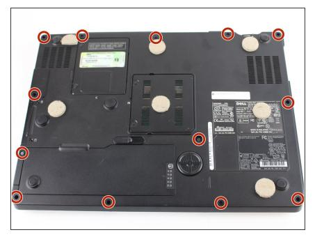
Remove the twelve 6mm Phillips case screws from the bottom of the case.
