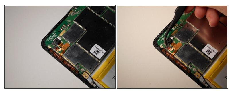
• The volume button assembly is in the top left corner of the tablet. To begin, you will have to pull the small black tab of the ZIF connector, shown in the second picture, to be able to remove the assembly. The tab is on a hinge so it should not be pulled off completely.
