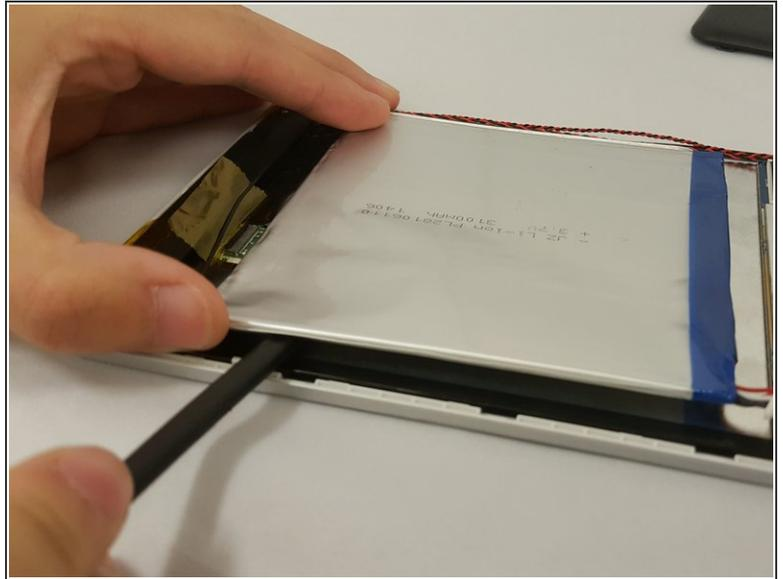
**⚠** Make sure to not bend or puncture the battery when removing it.
