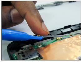
Using the blue spudger/prying tool remove antenna connectors by prying them up from the motherboard.
