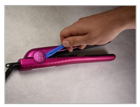
Use your fingers or a plastic opening tool to open the side hinges on both sides of the device.
