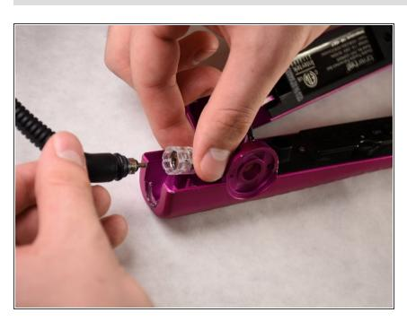
To remove the power cable, grab the clear plastic holding and the base of the power cable and pull apart. To reassemble your device, follow these instructions in reverse order.
