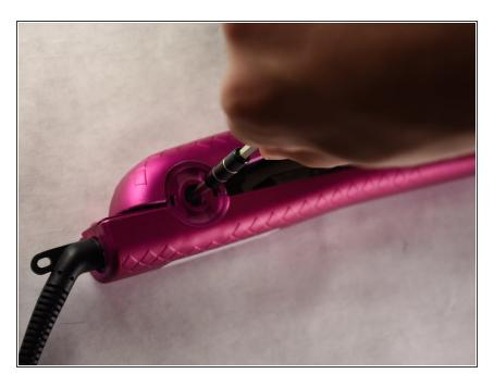
Using a Philips head #2 screwdriver remove the 7mm black screw from the hinge of the device.
