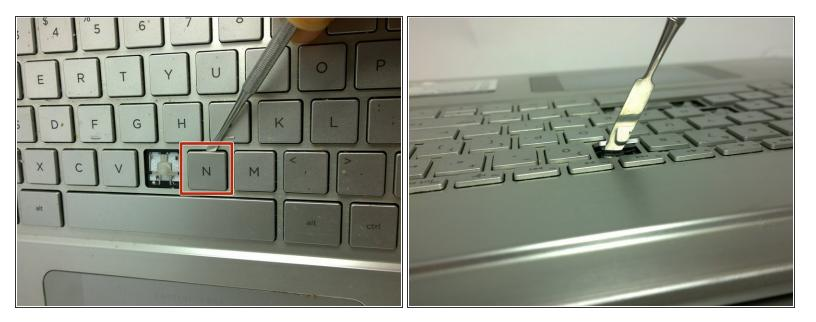
Use a metal spudger to separate key from keyboard.
