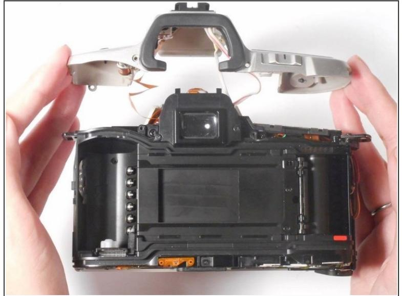
**i** The top panel of the camera should now be easy to pop off. If it is not, make sure that all screws listed in steps 3-9 are removed.
