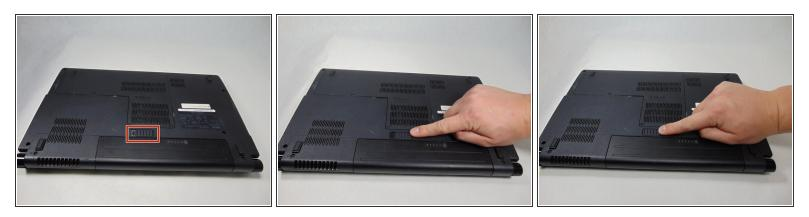
• Slide the locking switch to the left to release the battery.
