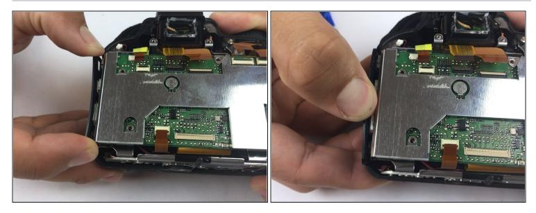
• Gently pull out the side wall of the camera so that the motherboard comes out easier.
