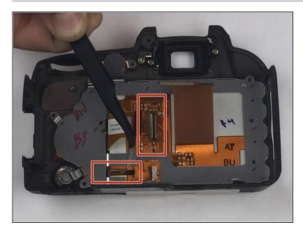
Remove the two ribbons connecting the LCD screen to the metal plate using the same method from Step 5.
