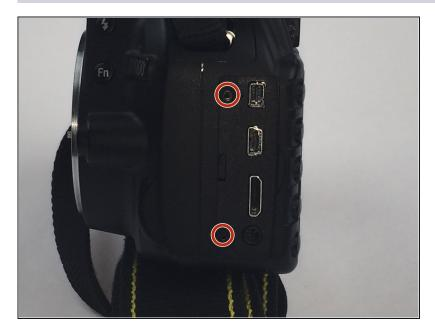
• Remove two of the 4mm screws on the left side of the camera.
