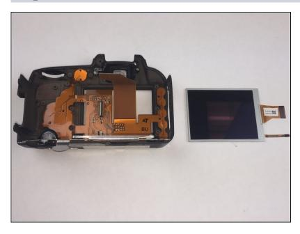
• Remove the old LCD screen from metal plate.
