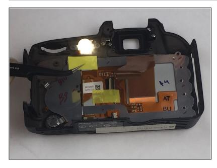
A Remove the tape covering the ribbons. Be careful not to break the tape.
