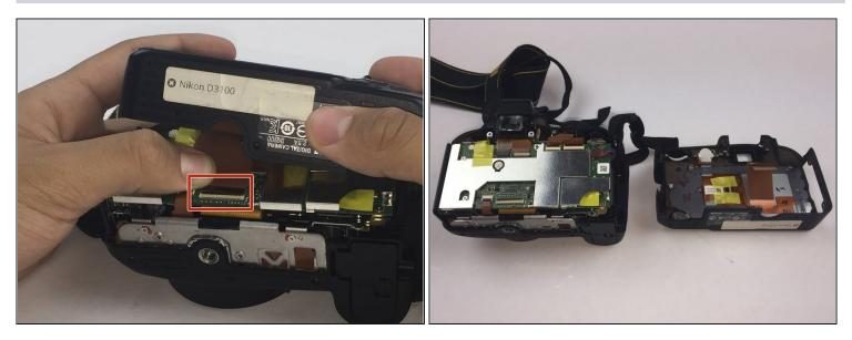
• Starting from the top, gently lift the back panel of the camera off. Slowly separate the back panel from the main body of the camera.
