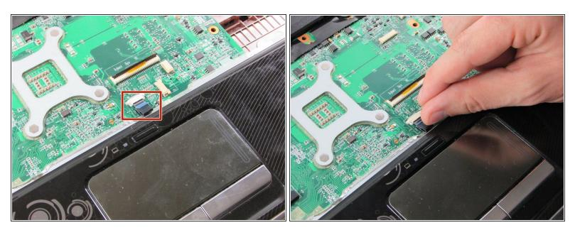
Disconnect the touch pad ribbon cable from the system board by gripping and pulling the blue tab toward you.
