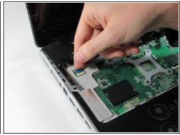
• Disconnect the LED board and power button cables from the connector on the system board by pulling the blue Mylar tabs toward the display screen.
