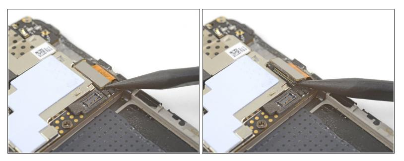
Use the point of a spudger to pry up and disconnect the display connector from its socket on the motherboard.
