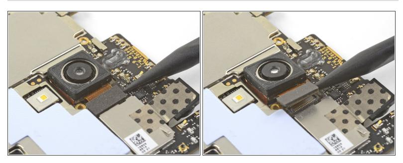
Use the point of a spudger to pry up and disconnect the rear-facing camera connector from its motherboard socket.
