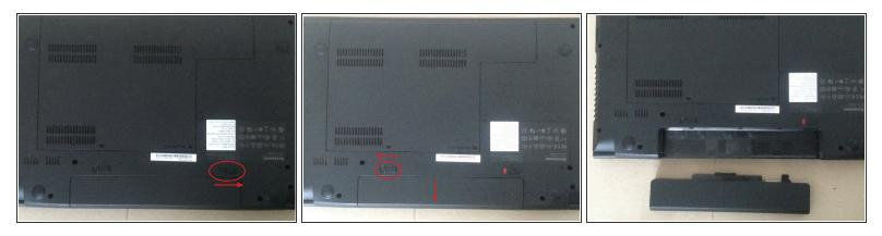
• Pull right trigger and unlock the battery.
