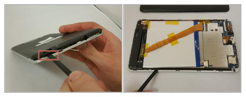
$\bigwedge$  Do not use a lot of force as it can break the clips or the back panel.
