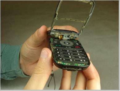
Once you have worked your way around the perimeter of the phone, you will have access to the components in the bottom half assembly.
