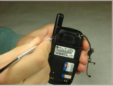
Remove the rubber covers in the highlighted locations using a metal spudger.
