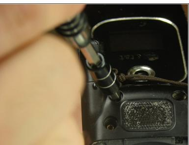
Remove the six 3mm #000 flat Phillips head screws from the back of the phone using a Phillips #000 Screwdriver.
