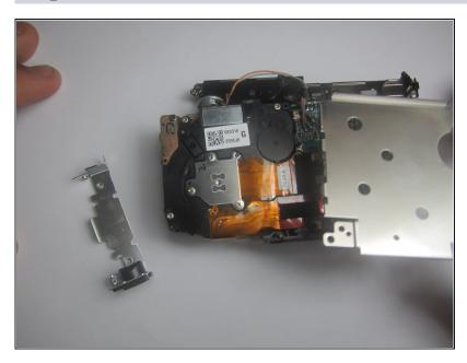
• Separate the two metal body pieces from the rest of the camera.
