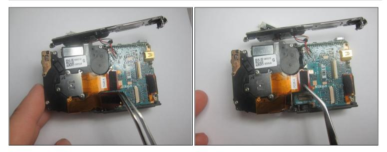
• Gently remove the two ribbons connecting the lens to the mother board.
