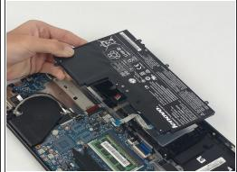
Gently lift the battery and use the plastic opening tool to remove the battery's connection to the laptop.
