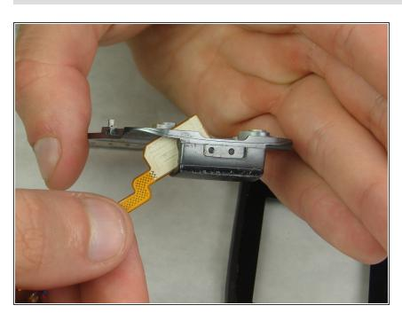
Carefully slide the display flex cable out. To reassemble your device, follow these instructions in reverse order.
