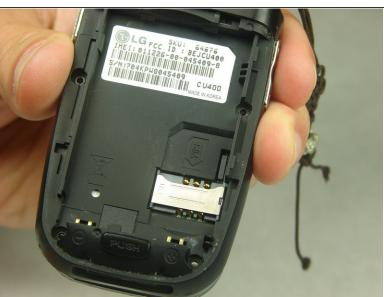
Remove the sim card by sliding the card out from under the retainer using either your fingers or a spudger.
