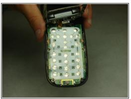
You should notice that the number pad is loose and can simply be taken out of the open phone casing.
