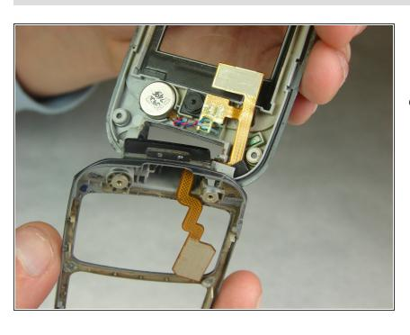
You can now carefully pull apart the phone casing at the hinge by separating them at the left side of the hinge.
