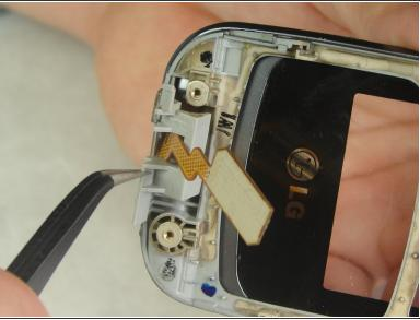
• Using tweezers, pull the gray plastic piece that is going around the flex cable out of the hinge area.
