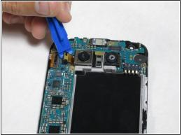
• Insert the plastic opening tool between the camera-ribbon connector and the motherboard, then pull up. It should pop out easily.
