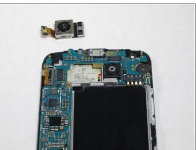
After detaching the ribbon, carefully remove the camera using tweezers
