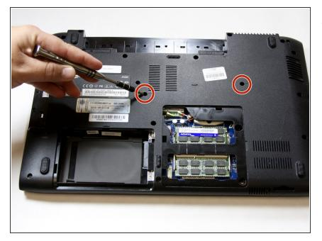
Remove the two 7mm Phillips head keyboard screws on the back plate labeled "KBD."
