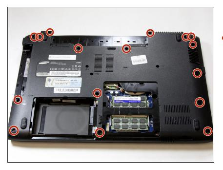
Remove the sixteen 9mm Phillips head housing screws on the back plate.
