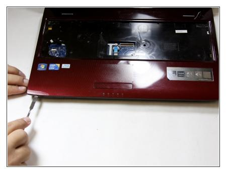
• Pry off the keyboard housing plate with the metal spudger and set aside.
