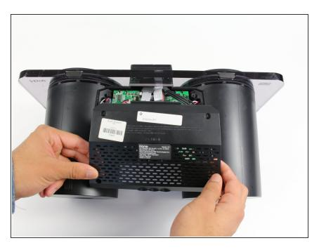
Remove the back cover by grabbing its sides and lifting it off the iHome.
