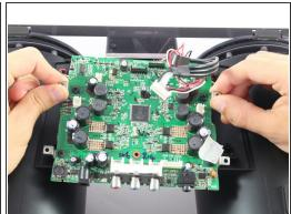
Remove the motherboard from its housing by grabbing it near its edges and carefully pulling it upward.
