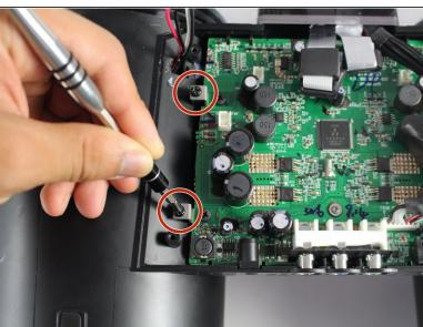
Unscrew the four 9.5 mm Phillips #2 screws on the four metal brackets located at each corner of the motherboard.
