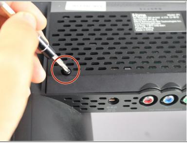
Remove the four 9.5 mm Phillips #2 screws located on each of the four corners of the iHome's back cover.
