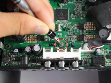
Unscrew the grey 6.0 mm Phillips #1 screw directly above the red, blue, and green component ports.
