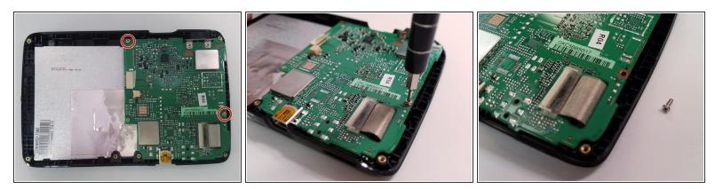
There will be two 5mm Phillips #00 screws that need to be removed from the motherboard.
