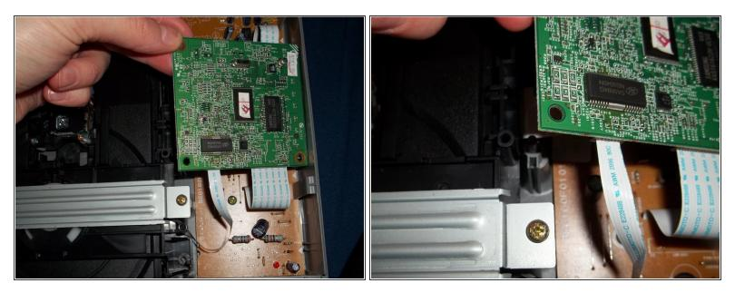
• Carefully lift the board just enough to remove the disk drive.
