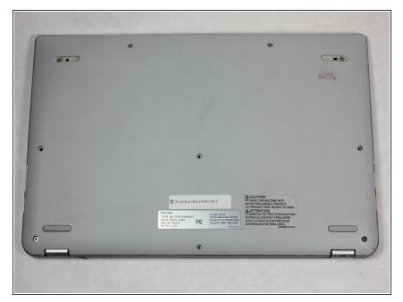
Close the Toshiba Chromebook 2 and turn it over so that the bottom of the laptop is facing upwards toward you with the lettering on the bottom facing right side up.
