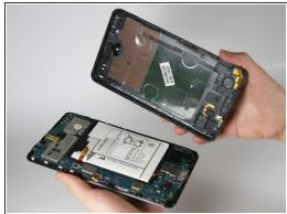
Carefully remove the back panel from the frame of the device.
