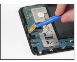
Disconnect the wire near the top of the motherboard by placing the plastic opening tool under the edge of the connector to flip it up.
