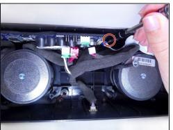
• Locating the two screws on either side of the motherboard, unscrew the two 8 mm Phillips head screws using a J1 Phillips head screw driver.
