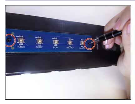
Place the device so the blue button panel is facing up, and use a J00 Phillips J1 head screw driver to remove the two 7mm Phillips head screws on either side of the button panel.
