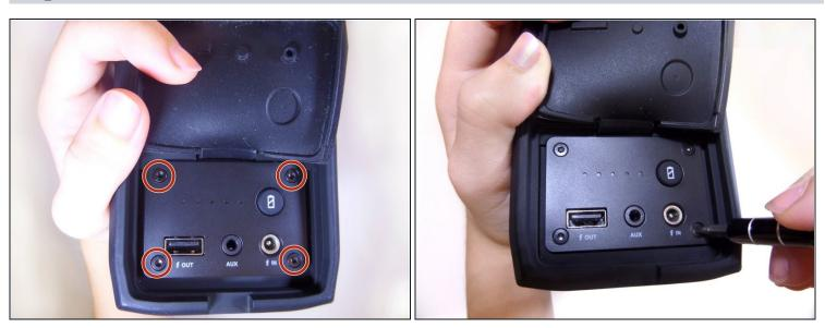
• Turning the device on its side, unscrew the four 15mm hexagon 2.0 screws on the charging port panel.
