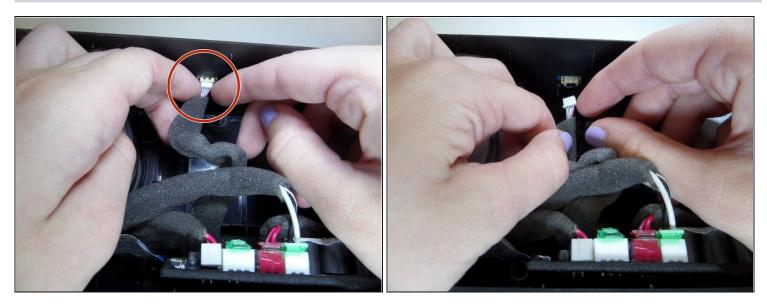
• Unplug the wire on the inside of the device that connect to the button panel.
