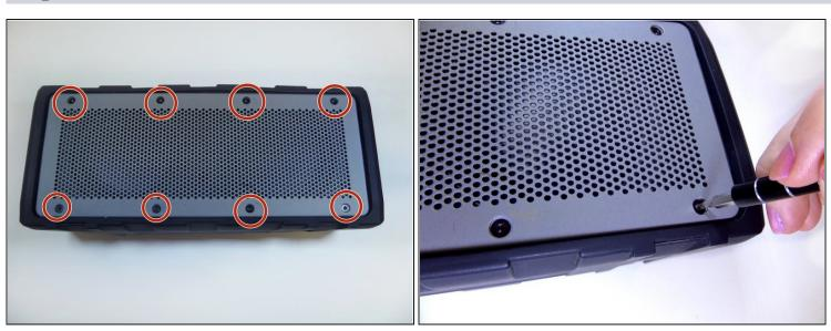
Placing the device with the back panel facing up, remove the eight 5mm hexagon 2.0 screws from the back panel.
