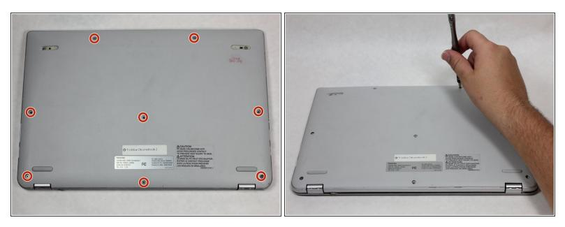
Remove the 8 visible Phillips 8.25 mm screws using the Phillips #0 screwdriver.
