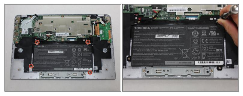
• Remove the 4 Phillips 2 mm screws holding the battery in place with the Phillips #0 screwdriver.
