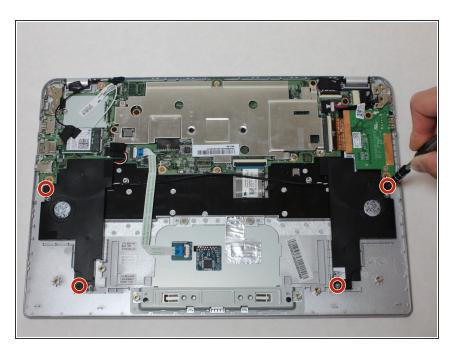
Remove the 2 3.3 mm screws holding the left and right speakers with the Phillips #0 screwdriver.
