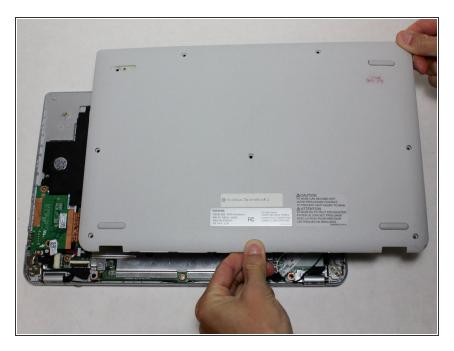
Remove the back panel by pulling up on 2 adjacent corners.
