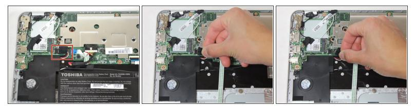
Pull the red and white wires out of the socket above the left speaker to disconnect the speakers from the motherboard.
