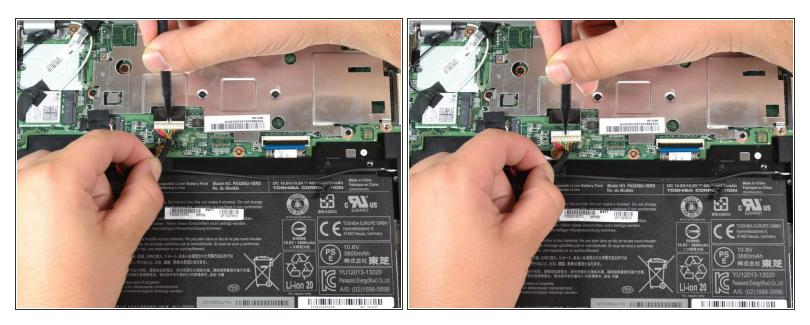
Press down on the white clip and softly pull the wires out of the port to disconnect battery from the motherboard.
