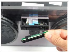
Remove the command buttons by pulling the small black panel containing them downward and away from the faceplate.
