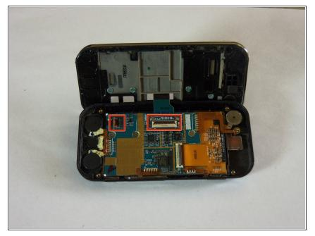
• After desoldering, verify that the gates on the two flex cables are in the "up" position and remove them.
