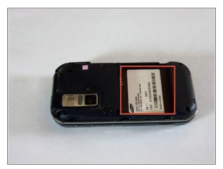
Remove the battery from the phone by using your plastic opening tool to find a gap at any edge of the battery and lifting the battery up.
