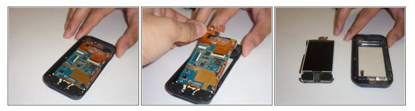
• Using gentle fingers, pry the LCD screen out of its housing.
