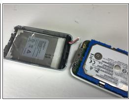
To detach wires from the screen, gently tug on the wires connected to the battery. They are located
