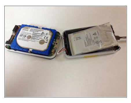
To begin removing the battery, move the wires out from under the black foam at the bottom of the device
