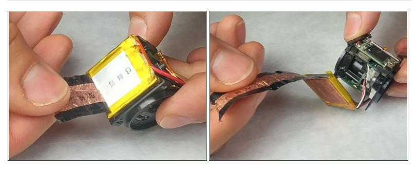
Remove the tape wrapped around the battery.
