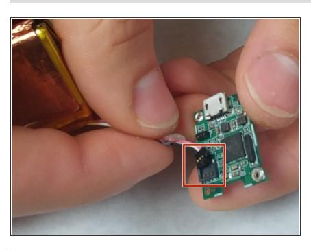
Gently remove the battery pin connector from the circuit board.
