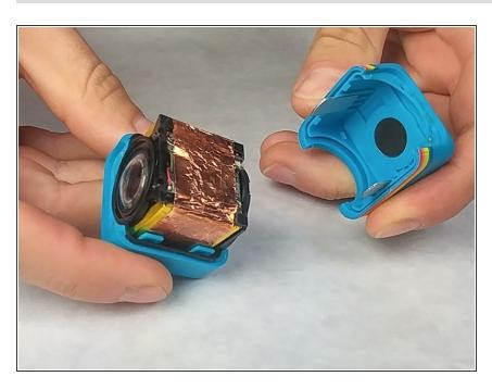
Remove shell from top and bottom of camera.
