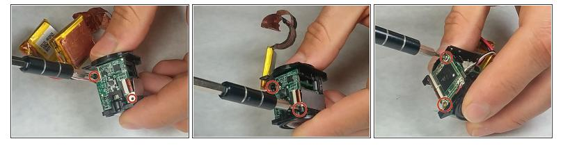
Using a J00 head screwdriver, unscrew the four 3.46mm screws from the top and bottom circuit board.
