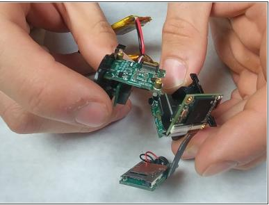
Use the plastic opening tool to remove the circuit board that the battery is connected to.
