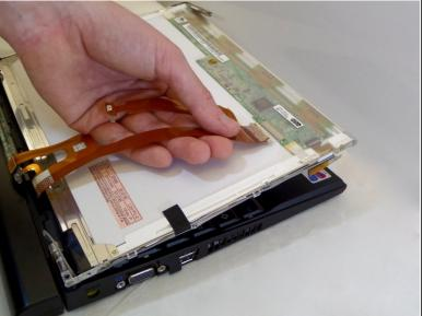
• Carefully disconnect the orange cable from back of LCD screen.
