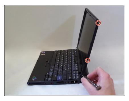
Using a Phillips Screw Driver, remove the (6) Phillips Head (Size PH001) 3.0 mm length screws (3 on each side) from the side of the LCD Screen Cover
