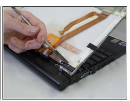
• Using a spudger, remove the black, rectangular support tape.
