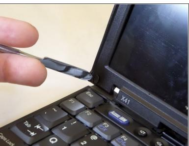
Using the spudger, remove the two round, black screw coverings on the lower, left, and right corners of the LCD screen bezel.
