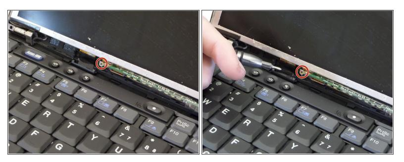
Use a Phillips head screwdriver to remove the internal LCD screen support assembly above the F6 key.
