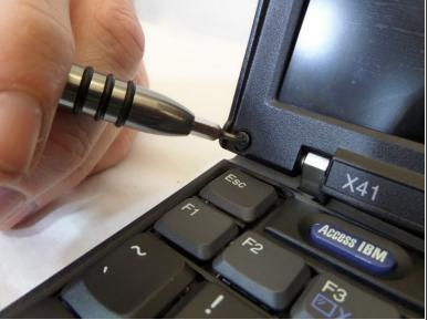
Using a Phillips Screwdriver (Size PH001), remove the 3.0 mm screws from the lower, left and right corners of the LCD screen Bezel
