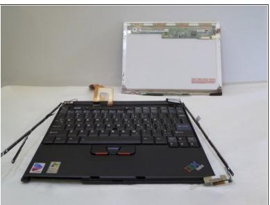
Using one hand, gently lift the LCD screen out of support arms.
