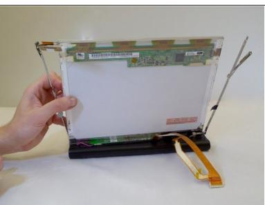
• Using a Phillips Screwdriver (Size PH001), remove the screws from the LCD screen support arms.
