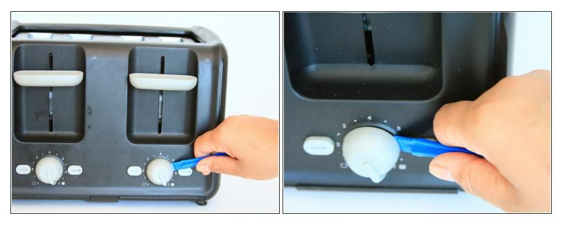
Pry the angled tip of a plastic opening tool behind the knob.
