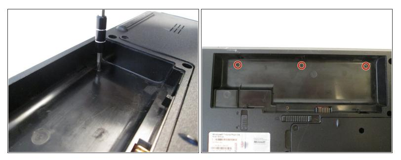
Use the Phillips #1 screwdriver to remove the three 4.5mm Phillips #1 screws.
