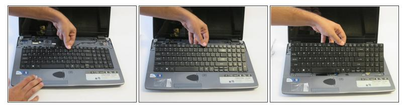
Insert a finger into the opening above the F11 key and pry the keyboard until it is released from the casing.
