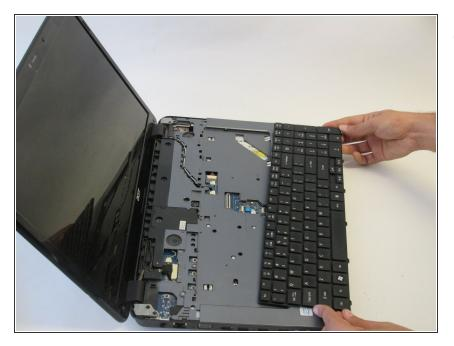
• Remove the keyboard from the keyboard slot.
