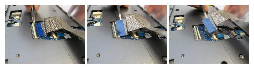
• Lift the black latch upwards to release the ZIF connector.
