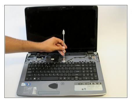
• Use the flat end of the medium sized metal spudger tool to release the two tabs at the top of the keyboard.
