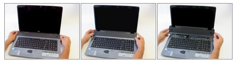
• Gently hold the speaker panel by the sides and pull upwards to release the panel.
