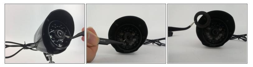
• Remove the foam ring around the lens with tweezers.
