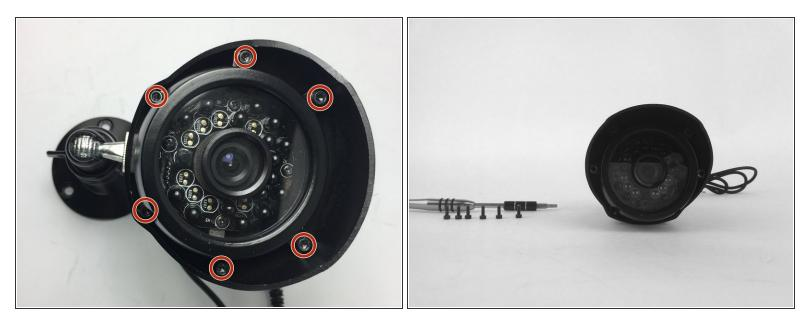
• Remove the six 10mm Torx T10 screws on the camera face.
