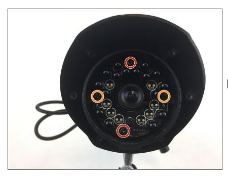
Remove the two 5mm Phillips #1 screws.
