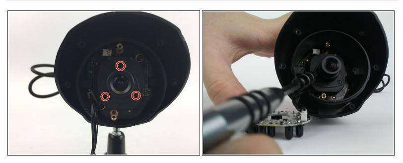
Use the Phillips #000 to remove the three 3mm screws on the face of the camera lens
