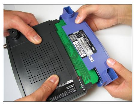
Squeeze the sides of the router's backcase inward and pull off the purple front case. It is helpful to have a second person assist you for this step.
