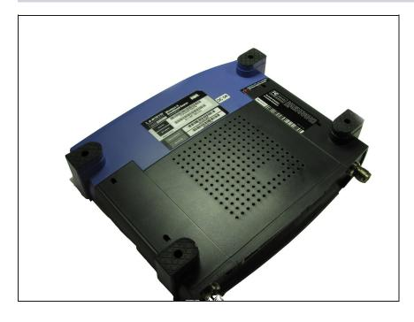
Turn the router over so that all four of its feet are facing upwards.
