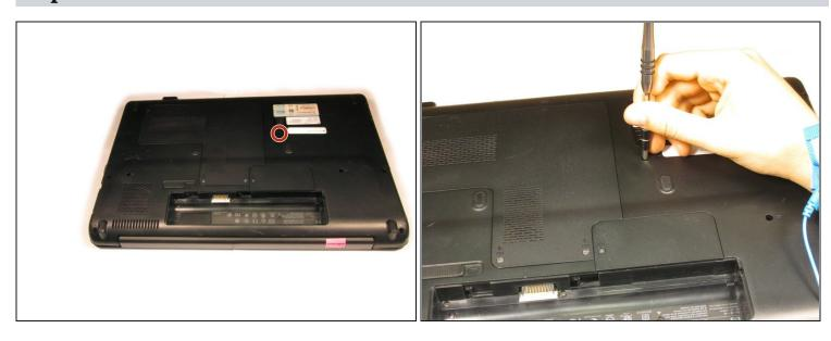
• Remove the 6mm screw above the laptop stickers using a Phillips #0 screwdriver.
