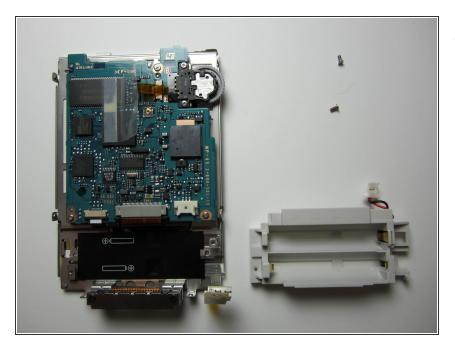
The battery harness is now removed. Install the new harness in reverse order.
