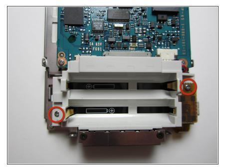
Remove the two screws holding the battery harness in place.
