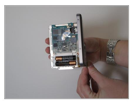
Remove the six screws holding the outer case.
