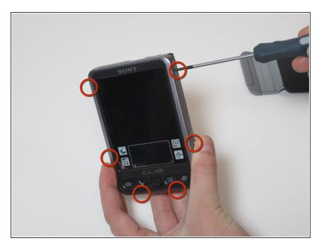
Remove the six screws holding the outside case of the Sony Clie.
