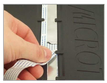
Grab the ribbon cable, and gently pull it off of the bottom of the scanner.
