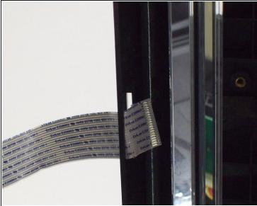
Simply remove the ribbon cable from within the holes it is wrapped through.
