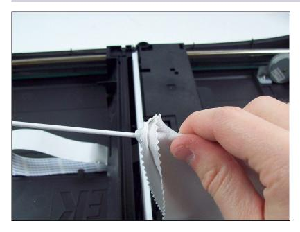
After opening the chassis and removing the bulb, simply take a cloth and wipe down the bulb.
