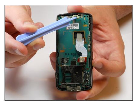
Using a plastic opening device, separate the top of the motherboard from the rest of the plastic casing.
