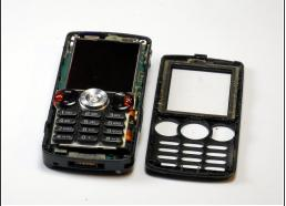
Run the plastic opening tool upwards along that side, removing the housing.
