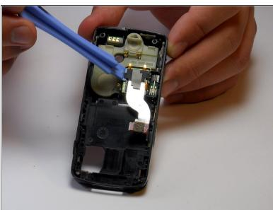
Push against the underside of the ribbon cable at the point of attachment with a plastic opening tool until it detaches.
