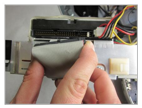
Flip the removed carrier to the right and pull out power cables.
