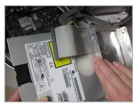
Slide the optical drive out of the carrier
