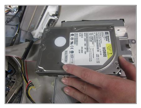
Slide the hard drive out from the frame and optical drive.
