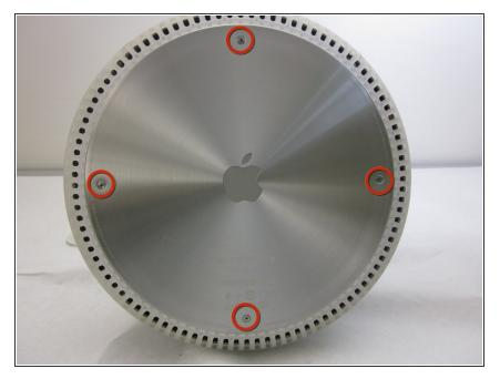
Loosen the four Phillips #0 screws.
