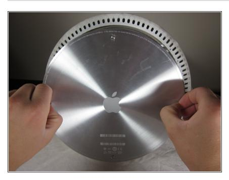
Carefully remove the base access panel.
