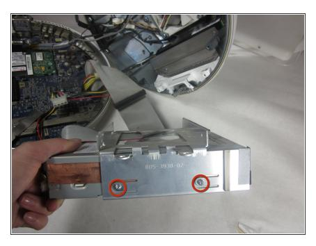
Remove the four T-10 6mm screws at the sides of the drive.
