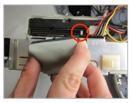
• Before you reassemble the computer, double check that your new hard drive has the same jumper configuration as the old one. This ensures the IDE "Master-Slave" protocol isn't interrupted. Some systems do not require this, but if you are having issues booting up afterwards with the storage or the disc drive, this could be the source of the problem.
