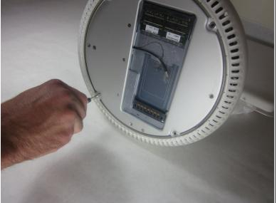
Remove the four 25mm T-15 screws.
